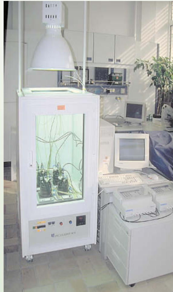
Laboratory system for measuring plants' oxygen output into their rhizosphere
