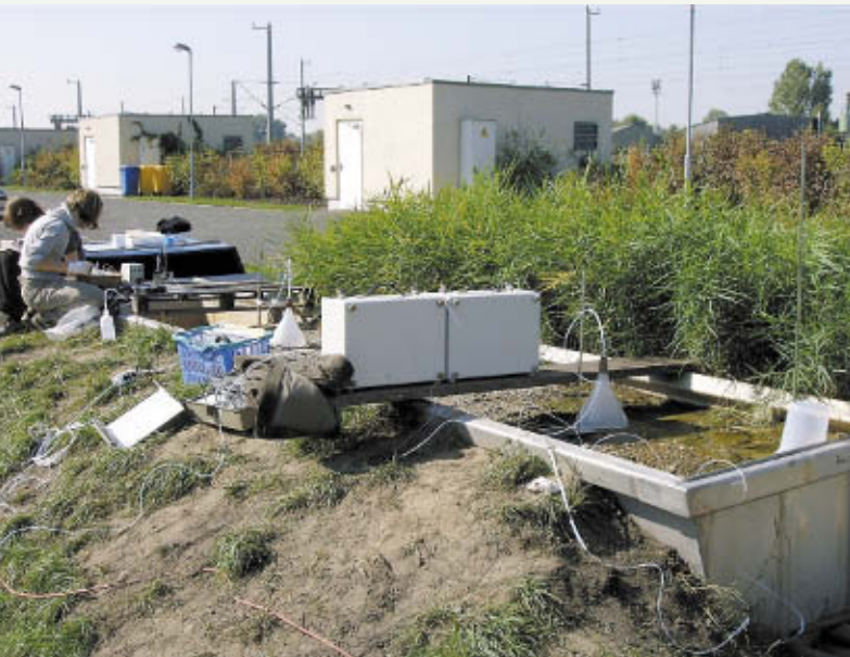
Meso-scale experimental wetland for groundwater remediation
