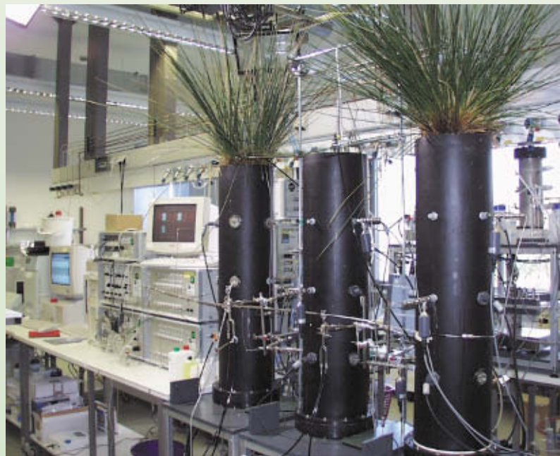
Column system to investigate nitrogen transformation processes
