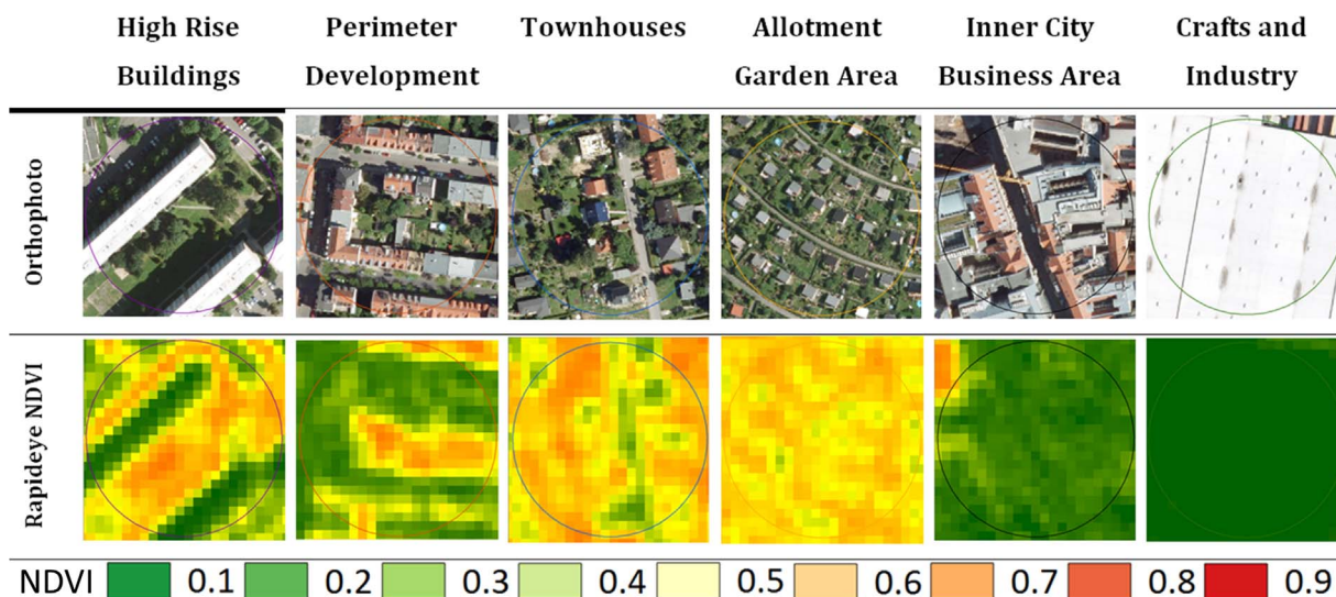
Fig. 6. Orthophoto and the corresponding NDVI values quantified by RapidEye data for urban built land use classes.
