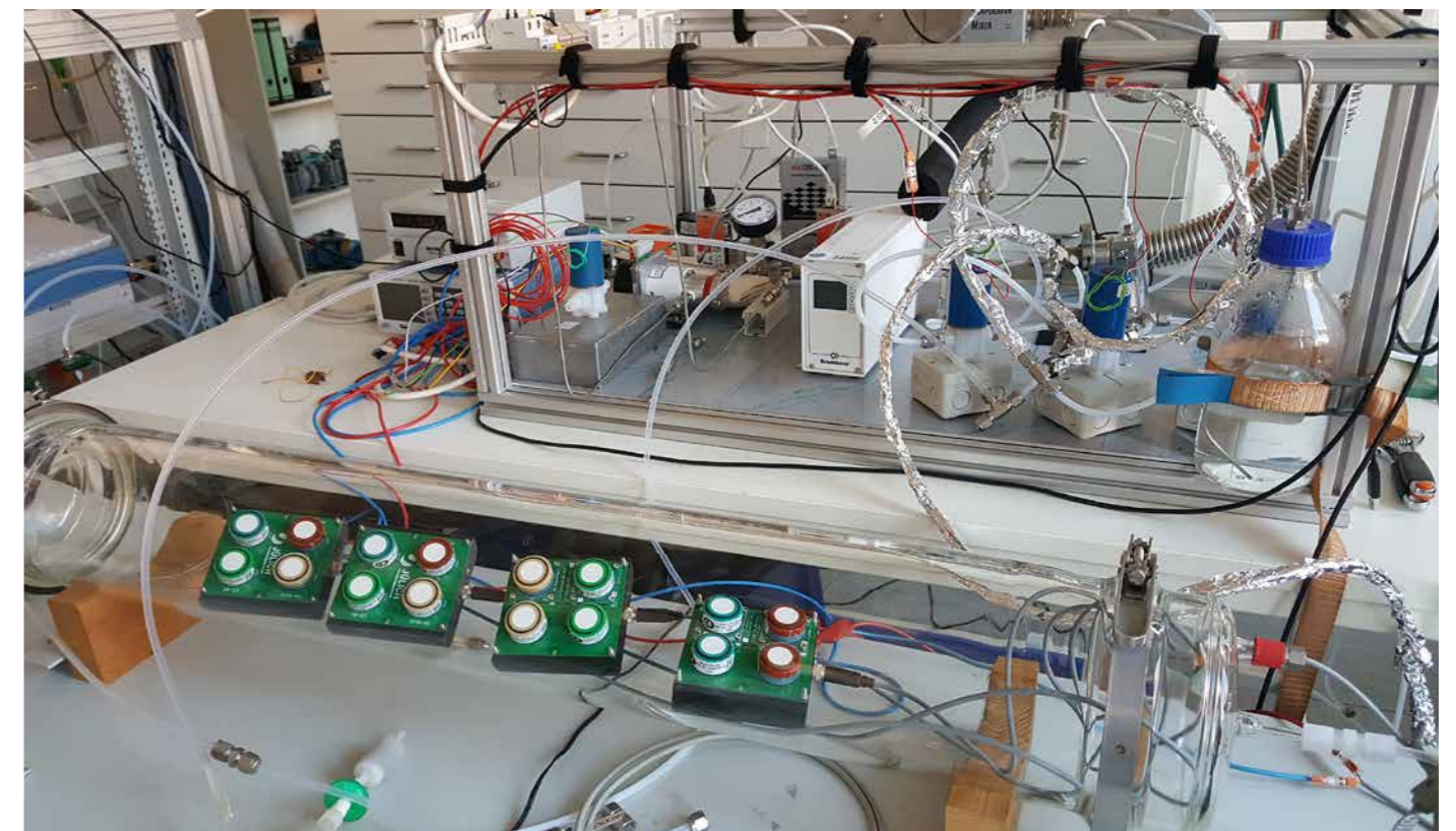
Calibration setup as part of the CS project SMARAGD (sensors for measuring aerosols and reactive gases and analysing their impact on health). Photo: Jülich Research Centre/Natalie Kille
