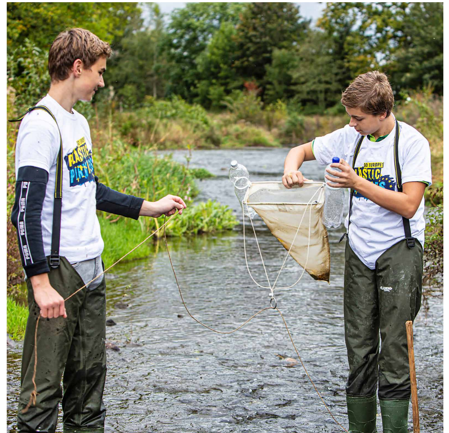
In full gear: participants in the campaign prepare to test the river for microplastics. To ensure that the data collected is comparable, the standardised special net is provided by the campaign. Photo: BMBF/Gesine Born
