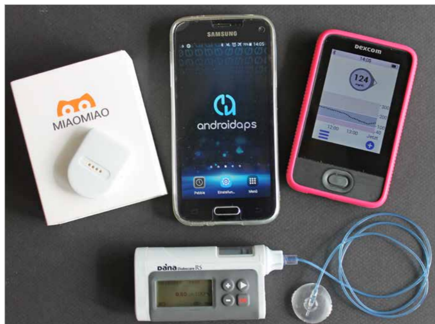
Components of an open-source closed-loop system of the TeQfor1 CS project. Photo: TeQfor1/KIT
