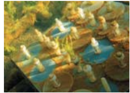
Substratum for biofilm growths that were exposed in a river.
