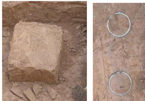
Figure 7: Extraction of tube sampling and block sampling at site Löbnitz:
