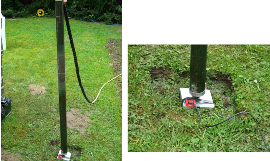
Fig. 5: SCPT source mounted in a 2 1/8" rod.
