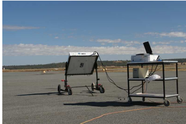
Figure 2-4. PLMR during cold point calibration orientated to the sky. The picture was made during another campaign in Narranda, Australia in December 2009.
