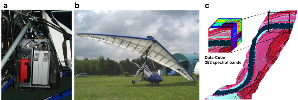
Fig. 3 a AISA-EAGLE (400–970 nm) and GPS/INS-RT3100 mounted on the UFZ’s microflight aircraft (Trike), b the UFZ’s microflight aircraft (D-MUFZ), c “Schleusenheger Wiesen” near Dessau recorded on July 3, 2008 with the UFZ’s microflight
